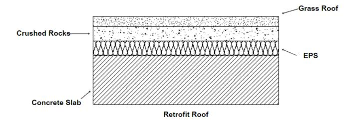
As this diagram shows, the added grass roof will sit on top of the crushed rock layer that is already present. The grass roof can be made of real grass or it can be astroturf, both will add a different amount of insulation while an astro-turf layer will be cheaper.
